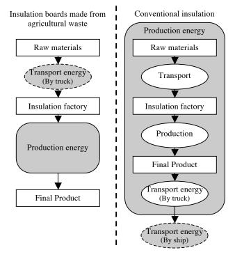
Figure 1: Flow chart identifying transportation and manufacture stages in the production of insulation boards made from agricultural waste in comparison with the production of conventional insulations.
